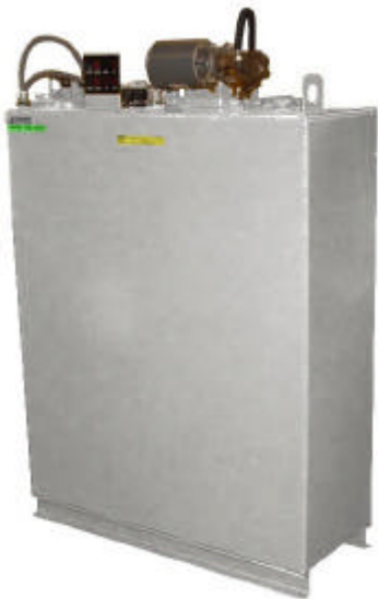
This is a 60-Gallon Trim, Double Wall, U/L Listed, Day Tank (PY60TULDW) without its cover. With cover, it is 61" tall, 42" wide. Its depth of only 16" includes the 3" double wall area that surrounds the inner tank.
